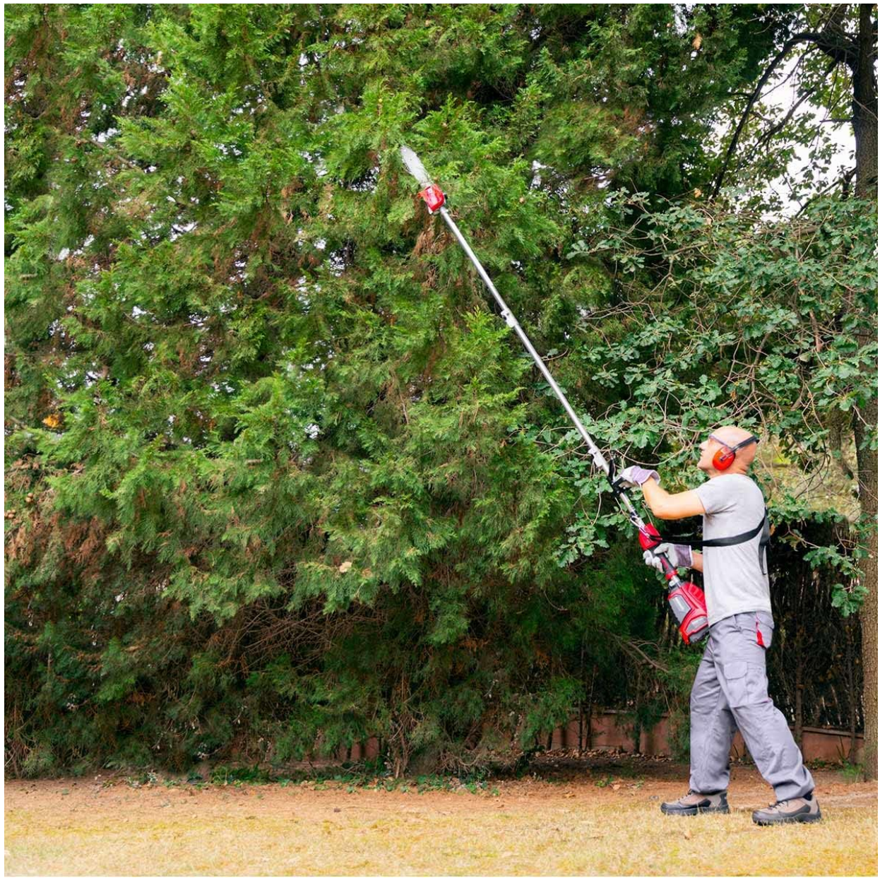
Figure 8: Operating the Pole Saw. This image shows a user safely operating the Greencut PP560L to prune high branches, demonstrating proper posture and reach.
