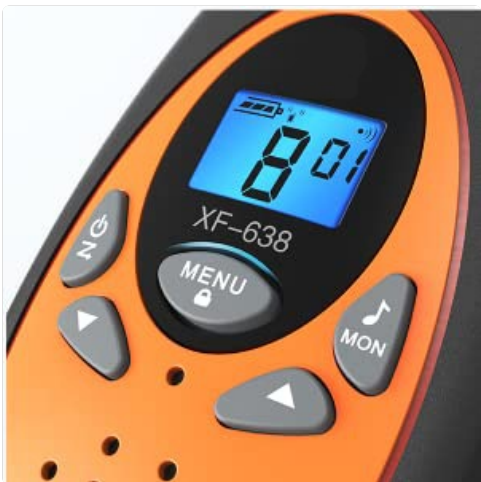
Image: Close-up of the walkie talkie's display and control buttons for channel selection.
