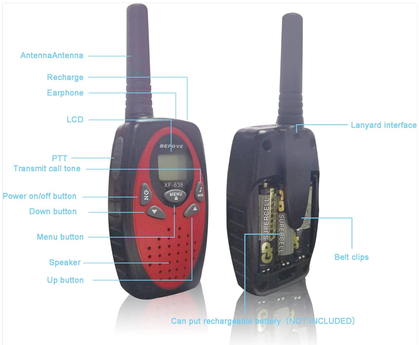
Image: Detailed diagram of the walkie talkie, illustrating battery placement and various components.
