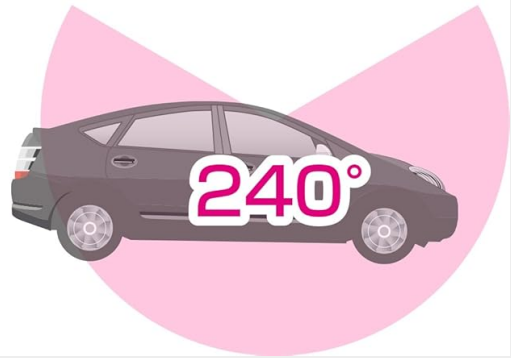
Image 2.2: Diagram illustrating the 240-degree vertical field of view, highlighting its ability to capture objects high above the vehicle.
