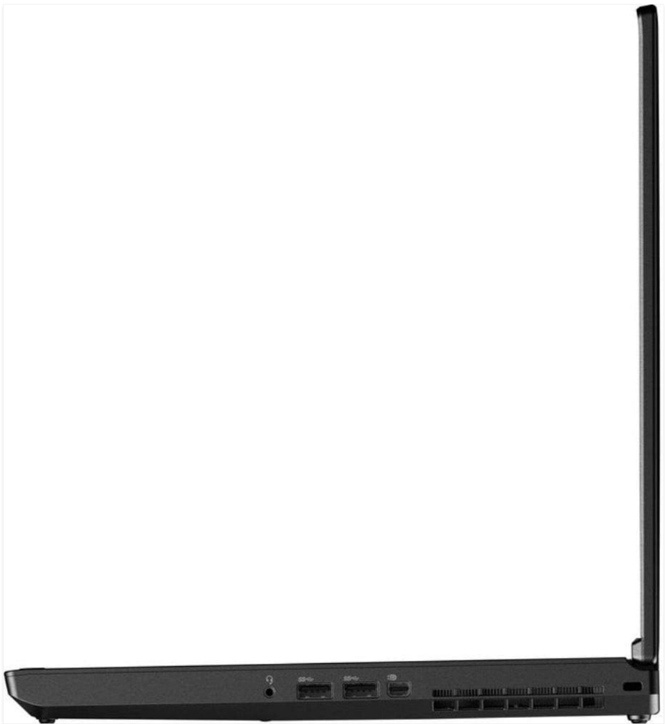
Figure 3.6: Right side ports of the ThinkPad P52, including additional USB ports.
