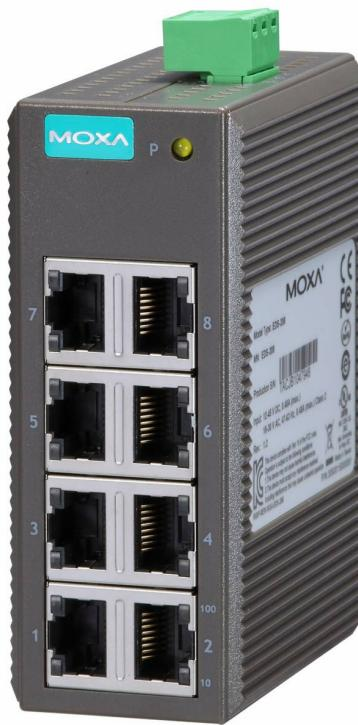
**Figure 1:** Moxa EDS-208 Unmanaged Ethernet Switch. This image displays the Moxa EDS-208 unmanaged Ethernet switch. The front panel features eight 10/100BaseT(X) RJ45 ports, numbered 1 through 8. Above the ports, the Moxa logo is visible, along with a 'P' indicator and a power LED. At the top, a green removable terminal block is present for power input. The device has a dark grey plastic housing with ribbed sides for heat dissipation.
