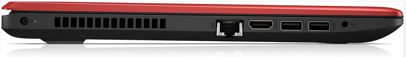
Figure 2: Left side of the HP 15-bs234wm laptop, highlighting the power input port.
