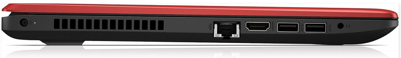
Figure 5: Left side of the HP 15-bs234wm laptop, showing the Ethernet, HDMI, and USB ports.
