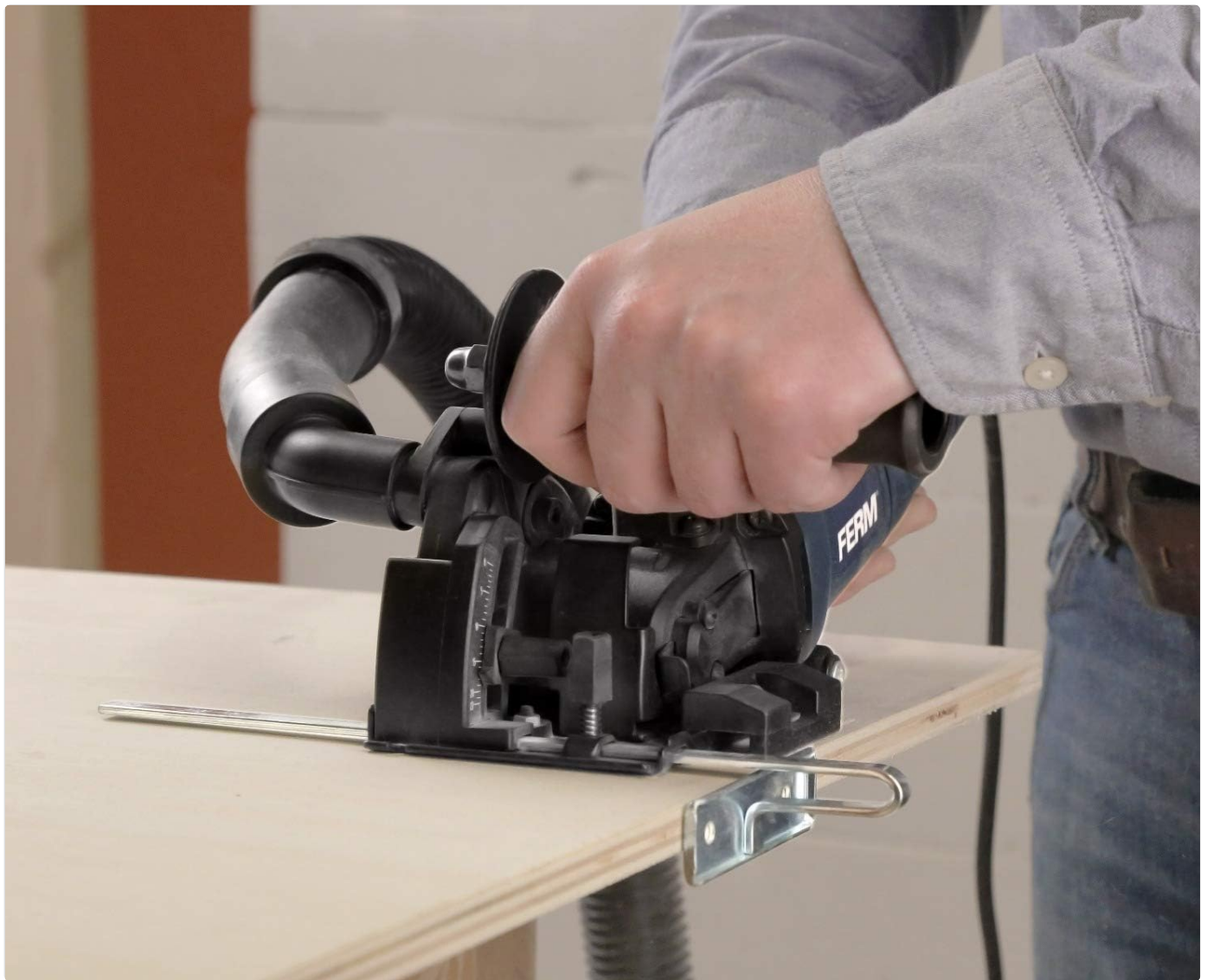
Image: A user utilizing the parallel guide with the FERM CSM1043 to make a straight cut on a piece of wood, demonstrating enhanced precision.
