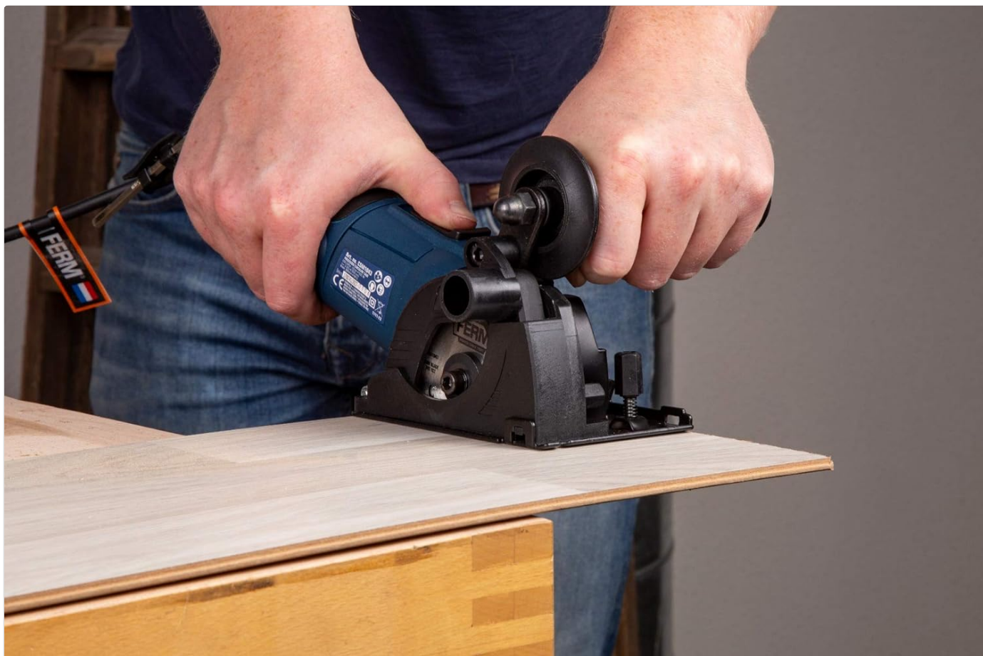
Image: A user cutting laminate flooring with the FERM CSM1043, showcasing its capability for common household and DIY tasks.
