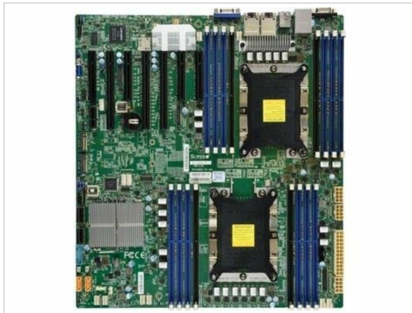
Figure 1: Supermicro X11DPH-I Server Motherboard overview. This image displays the general layout of the motherboard, including various slots and connectors.
