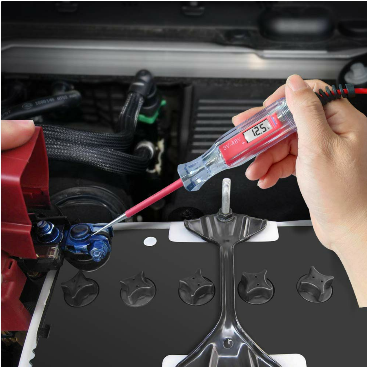
Figure 4: Demonstrating the test light in use, checking voltage at a car battery terminal.
