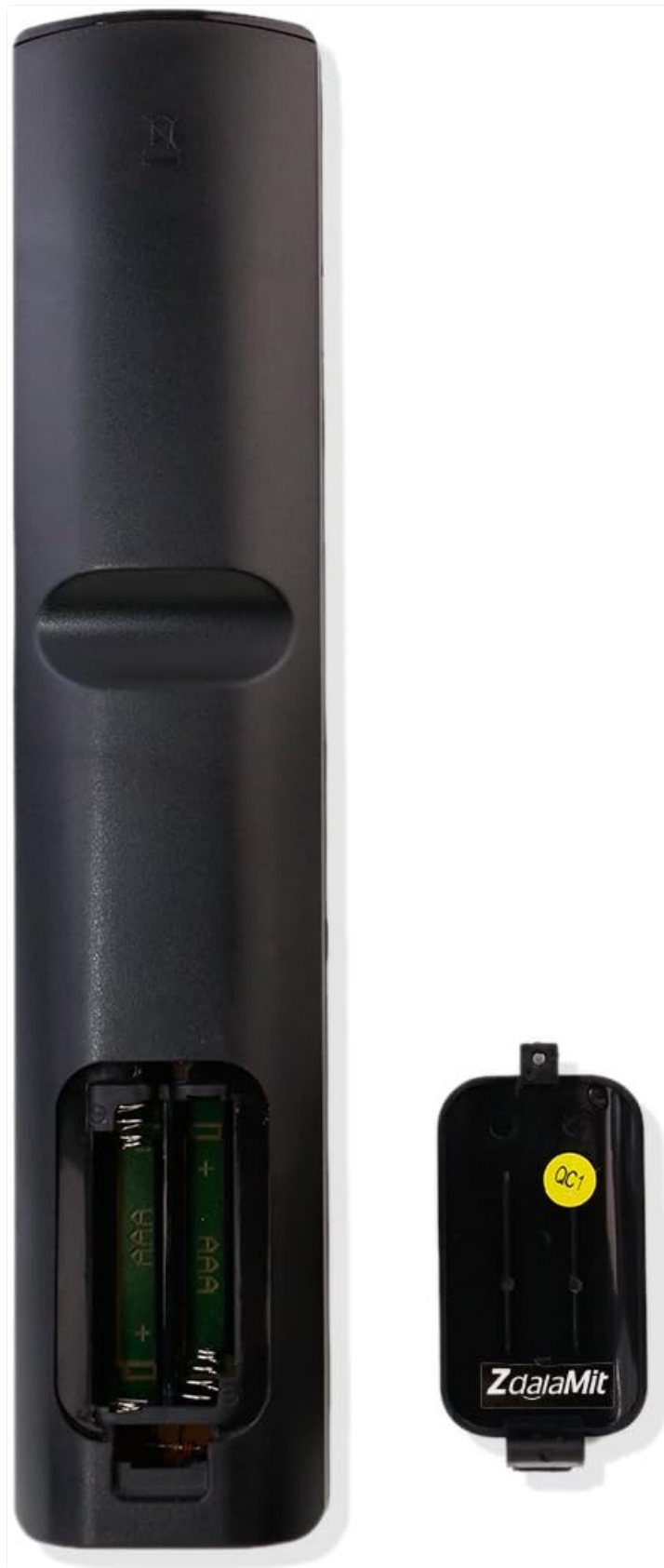
Image: Back of the remote control with battery compartment open. This image displays the rear side of the remote control, highlighting the battery compartment. The cover is removed, revealing two AAA batteries correctly inserted, indicating the proper orientation for battery placement.
