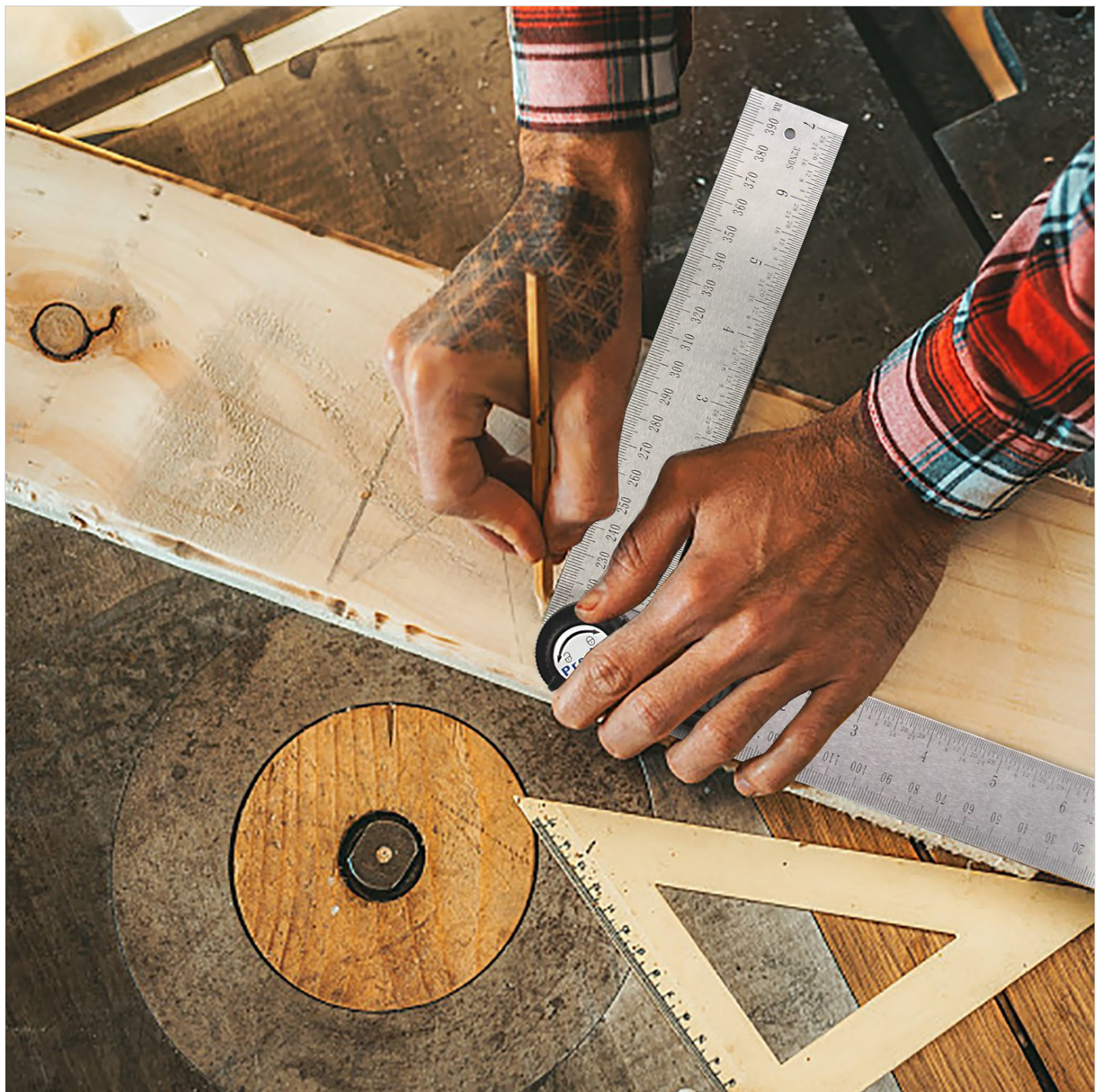
Figure 4.1: Using the angle finder to mark precise angles on a workpiece.
