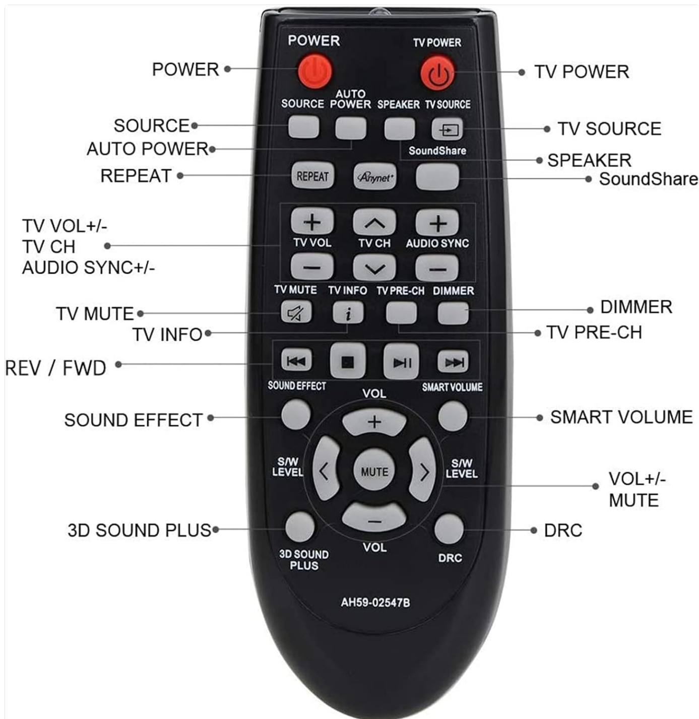
Figure 4: Labeled diagram of the remote control buttons.
