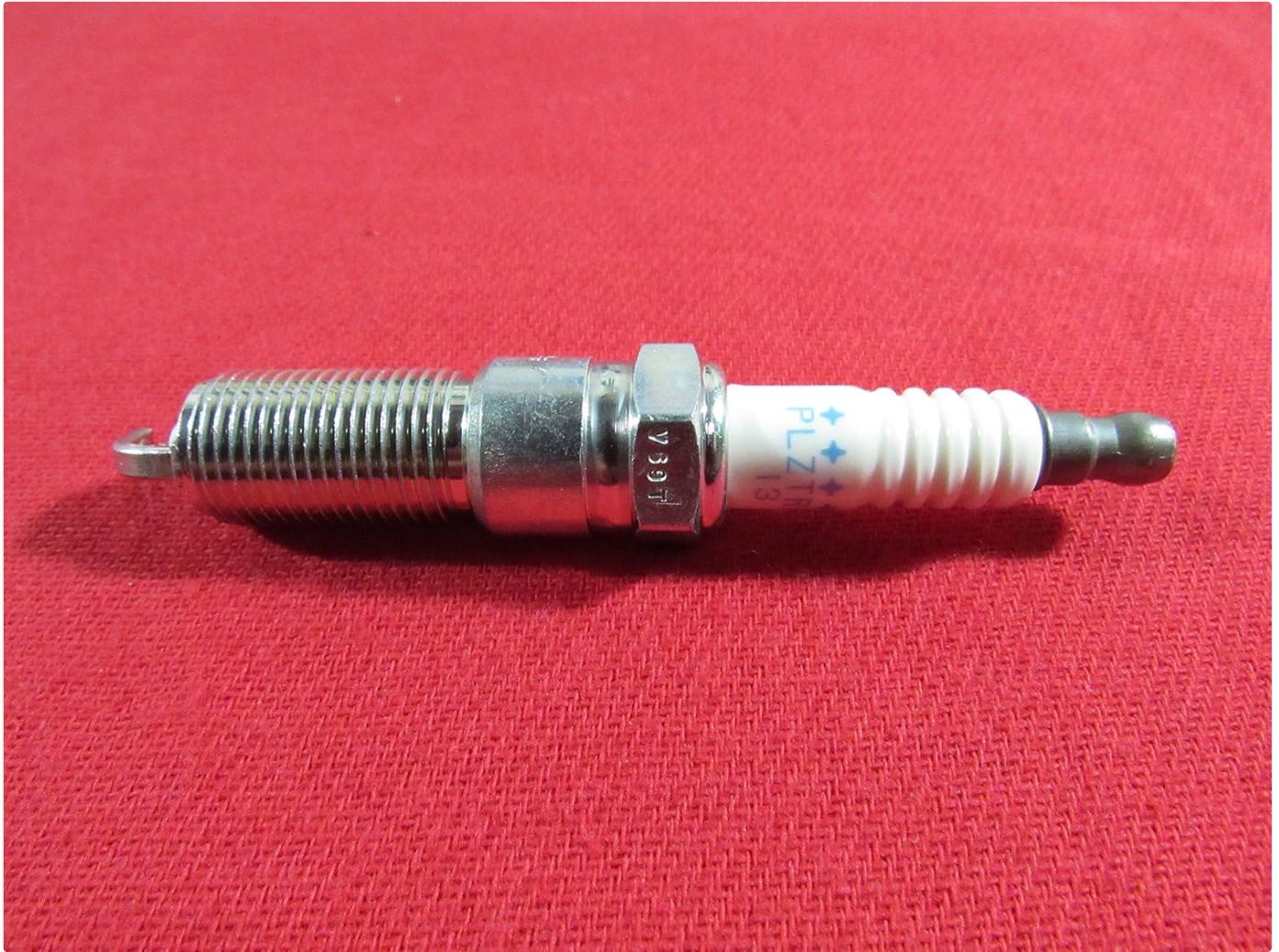
Image: A detailed view of a single Mopar spark plug, highlighting its ceramic insulator, metal shell, threads, and electrode tip. This view is useful for inspecting the plug before installation.
