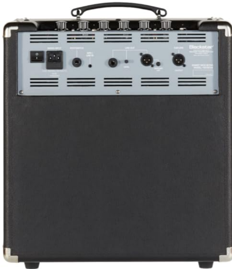
Figure 2: Rear panel connections, including Mains Input, Footswitch, MP3/Line In, Line Out, and Cab Link.
