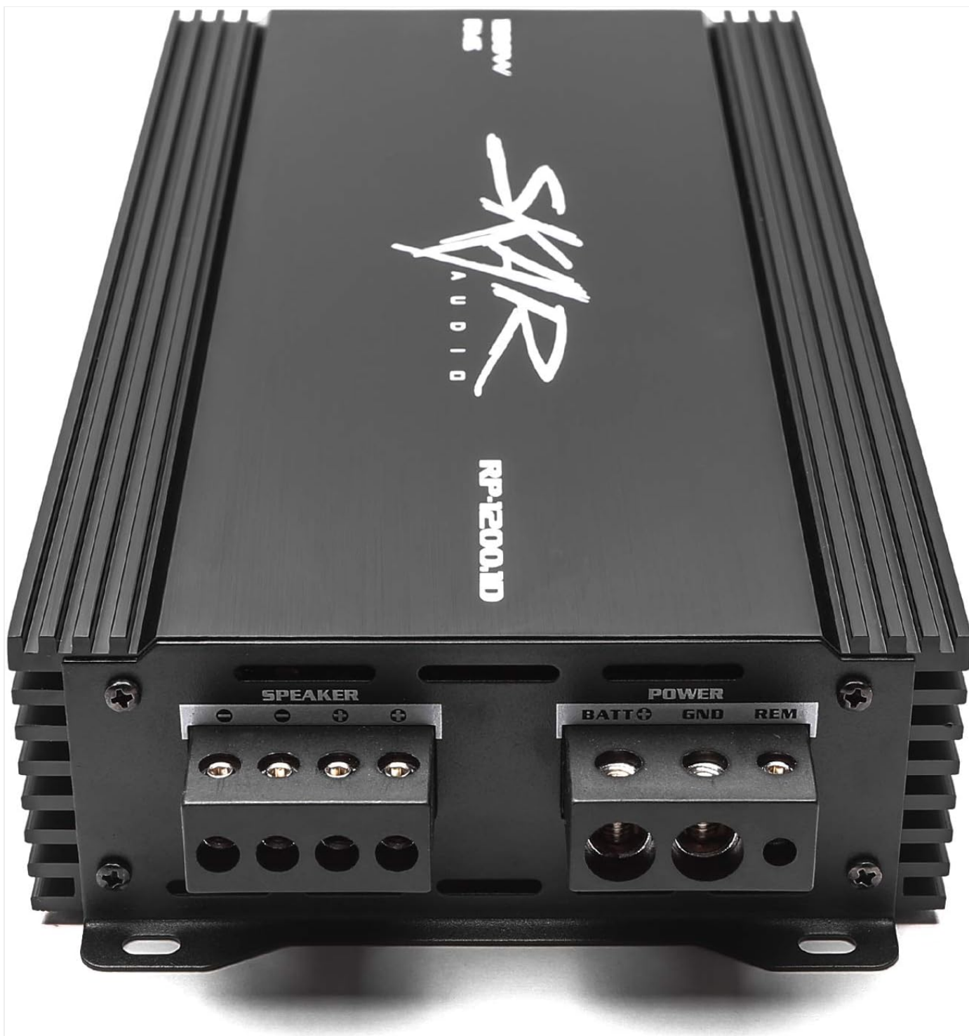
Figure 3: Power and speaker terminal side of the amplifier.
