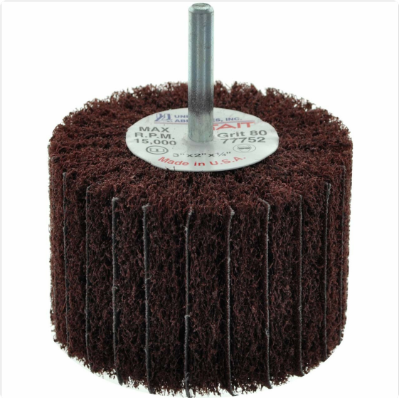
Figure 3.1: The SAIT 77752 Non-Woven Interleaf Wheel. This image shows the cylindrical abrasive wheel with its central arbor, ready for mounting onto a compatible power tool such as a die grinder. The wheel features multiple layers of abrasive material, indicating its interleaf construction.
