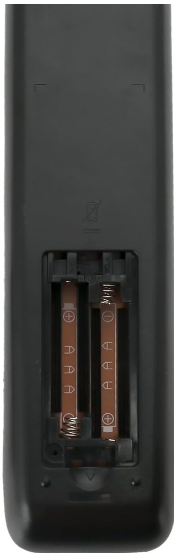
Image: Back of the remote control with the battery compartment open, illustrating the correct placement for two AAA batteries.
