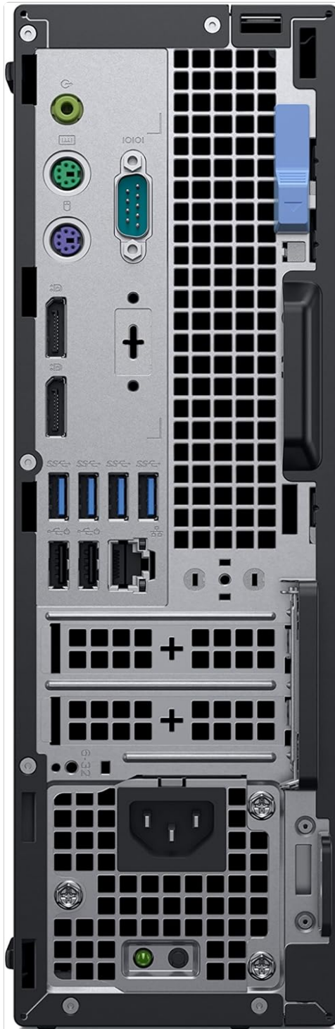
Figure 2.3.2: Rear View of OptiPlex 7060 SFF. This image illustrates the back panel, featuring display ports (DisplayPort, HDMI), multiple USB ports, Ethernet port, audio jacks, and the power connector.
