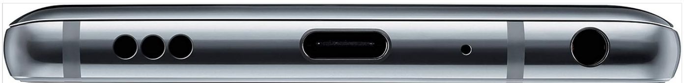
Figure 2.1: Bottom view of the LG G7 ThinQ, showing the USB-C port and 3.5mm audio jack, relevant for charging and audio accessories.
