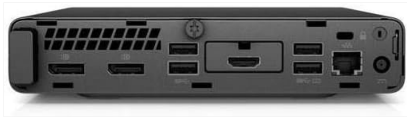
Figure 2.2: Rear panel of the HP ProDesk 600 G4 Mini, including DisplayPort, HDMI, multiple USB ports, and an Ethernet port.
