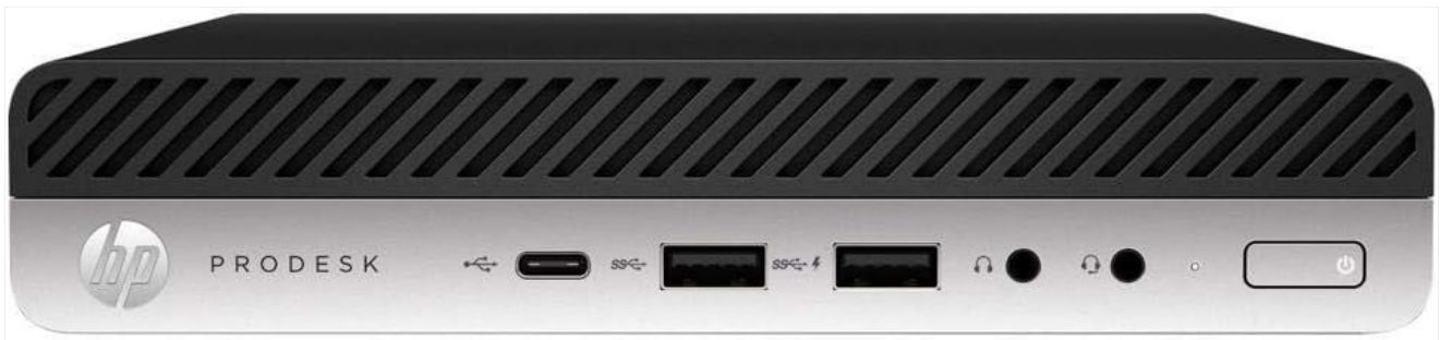
Figure 2.1: Front panel of the HP ProDesk 600 G4 Mini, featuring USB-C, two USB 3.0 ports, and audio jacks.
