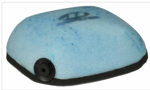
The Maxima Racing USA AFR-5007-01 Air Filter features a bonded dual-stage open cell foam matrix. The outer foam layer is 6 millimeters thick, and the inner foam layer is 10 millimeters thick, providing excellent filtration capabilities. The filter is pre-oiled with Maxima FFT filter oil, making it ready for immediate installation. Its high-strength glued seams ensure durability and longevity. Each package includes disposable gloves for convenient handling.
