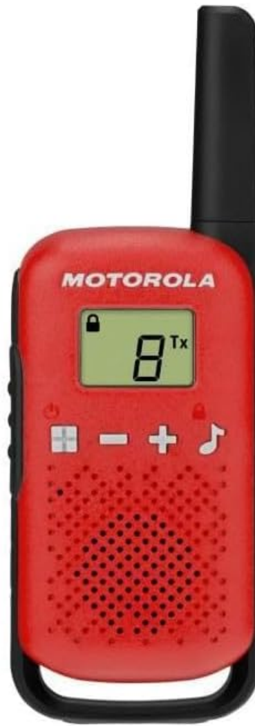
Figure 2.1: Front view of the Tlkr-t42 radio, showing the display, control buttons, and speaker grille.
