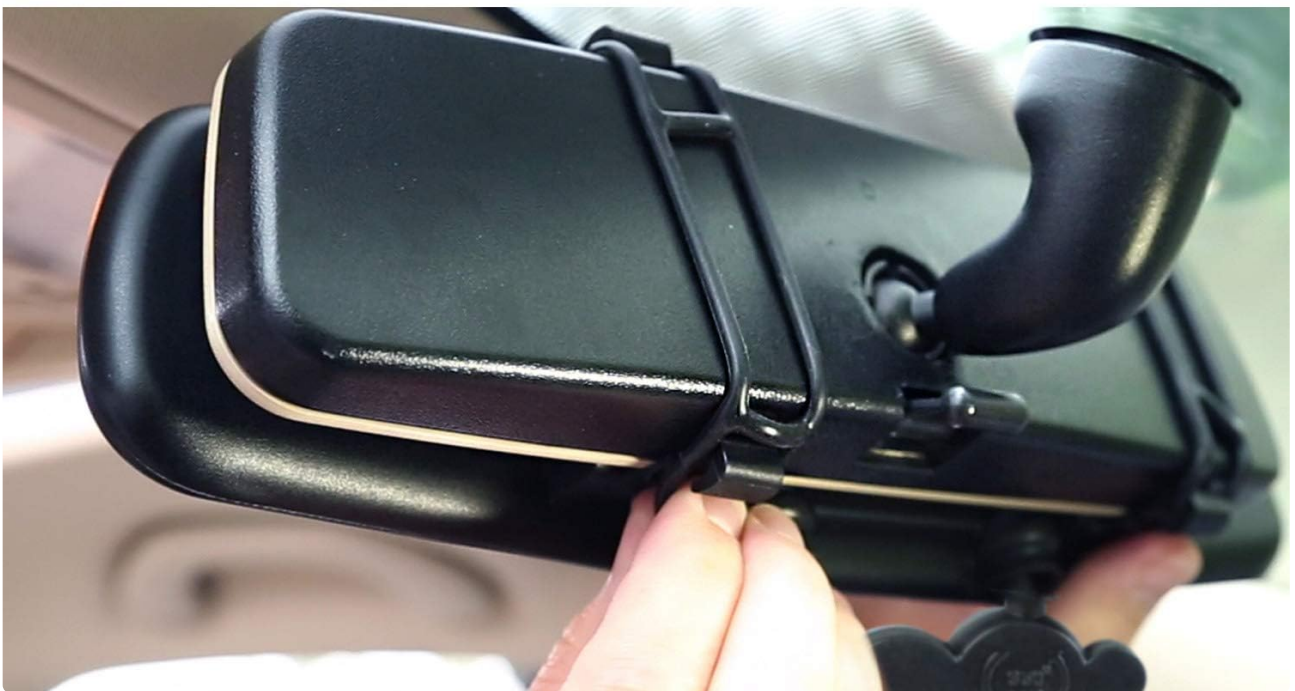
Figure 2: Installation of the HD Mirror Cam. The image shows a person attaching the dash cam unit over a vehicle's standard rearview mirror, demonstrating the use of the soft bands for secure fitting.
