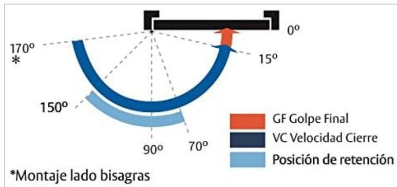
**Image Description:** This diagram details the operational angles of the door closer, including the final closing stroke (GF Golpe Final), closing speed (VC Velocidad Cierre), and retention position (Posición de retención). It shows how the door's opening angle affects these settings, with a retention point indicated between 70 and 150 degrees, and the final closing action from 15 degrees. The asterisk indicates 'Montaje lado bisagras' (hinge side mounting) for the 170-degree maximum opening.
