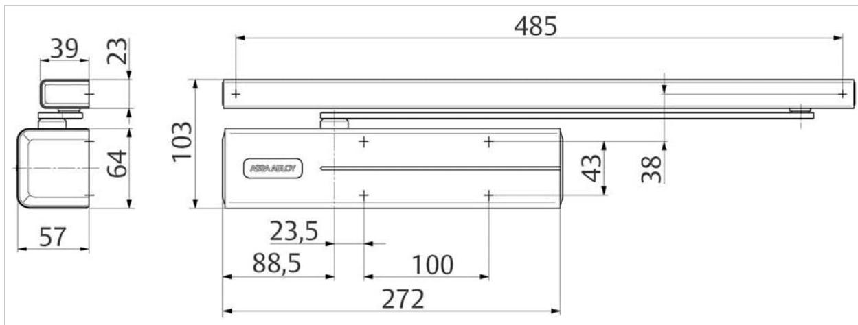
**Image Description:** This diagram illustrates the precise dimensions of the Tesa Assa Abloy DC700 door closer body and its associated sliding arm. All measurements are provided in millimeters, crucial for accurate installation and pre-drilling. Key dimensions include the overall length of the arm, the height and width of the closer body, and the spacing for mounting holes.
