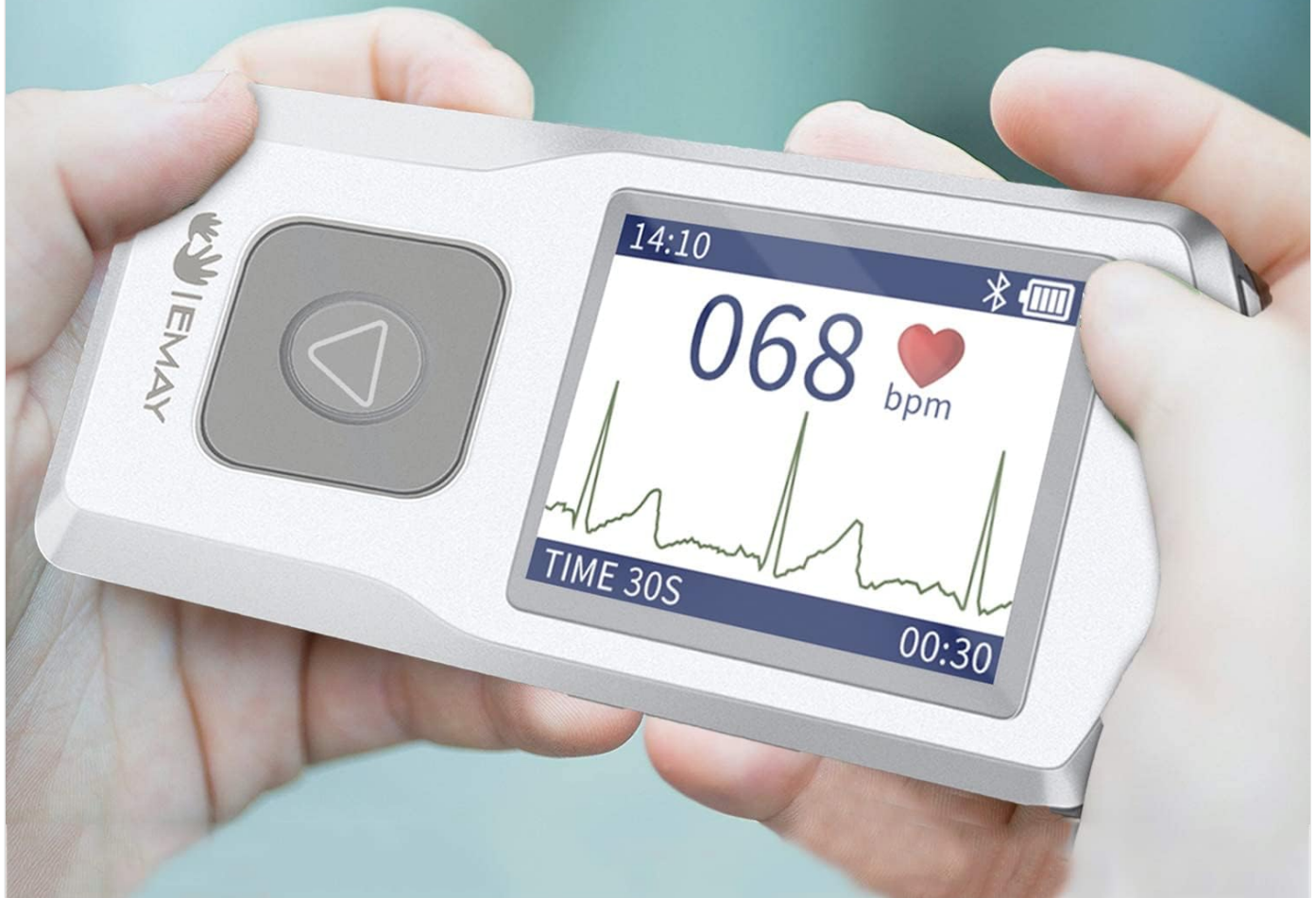
Figure 4: Stand-alone EKG device with real-time display.
