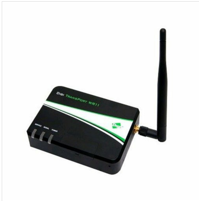
Figure 1: Front view of the DIGI WR11-L800-DE1-SU Wireless Router. This image displays the compact design of the router, highlighting the various ports and LED indicators. Visible components include the power input, Ethernet port, and antenna connectors. The status LEDs provide visual feedback on power, cellular signal strength, and network activity.
