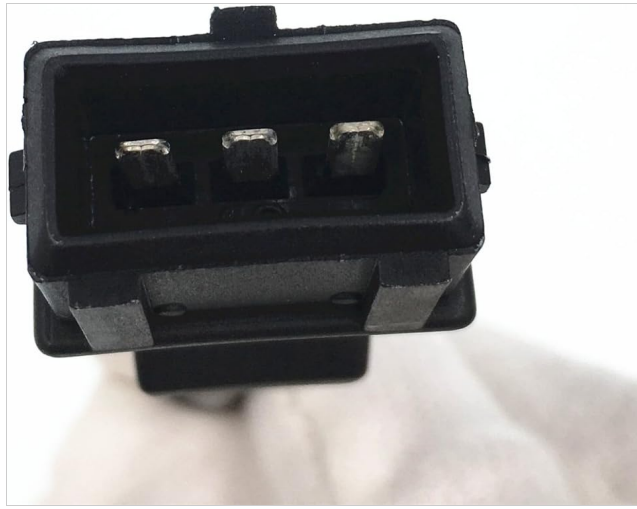
Image 4: Detailed view of the electrical connector pins. This shows the contact points for the vehicle's wiring, which should be clean and free of corrosion for proper signal transmission.
