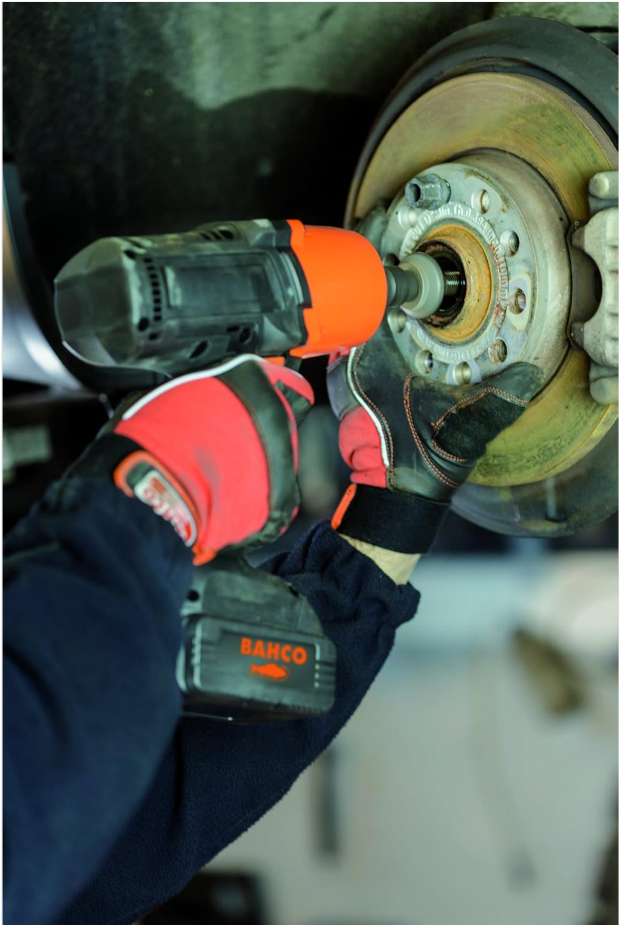
Figure 4.1: User operating the Bahco BCL331W2 Impact Gun to work on a vehicle's wheel assembly. The image shows the tool being used in a practical application, demonstrating its ergonomic design and ease of handling.
