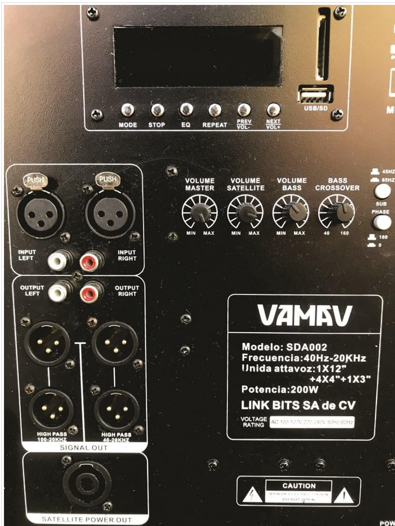
Image: A close-up view of the control section on the Vamav AURAL SDA002 subwoofer's rear panel, highlighting the volume, bass, and crossover knobs, along with input/output ports.
