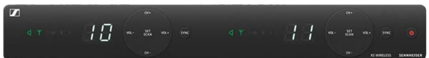
Image: Front panel of the receiver showing channel displays, volume controls, scan, and sync buttons for both channels. The front panel features two independent channel displays, volume controls, and 'SET/SCAN' and 'SYNC' buttons for each channel. These allow for easy frequency scanning and synchronization with the transmitters.
