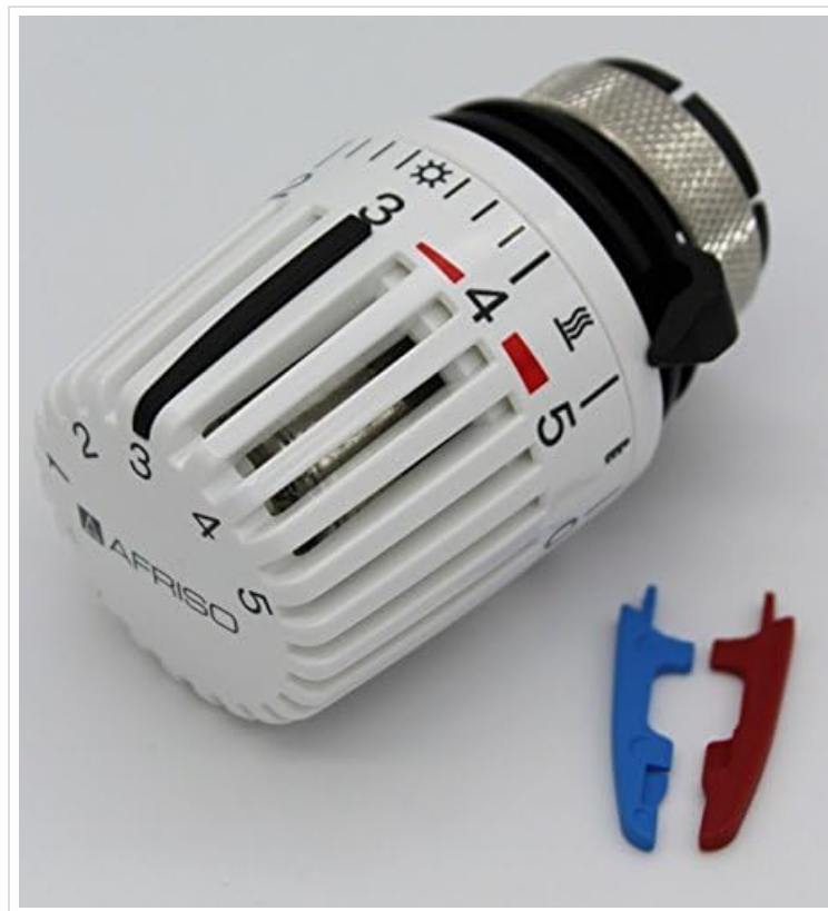
Figure 1: The Afriso Thermostatic Radiator Head Type 320 N, showing the temperature scale (0 to 5, with snowflake and wave symbols) and the Afriso logo. Two small red and blue plastic clips, used for limiting the temperature range, are also visible.
