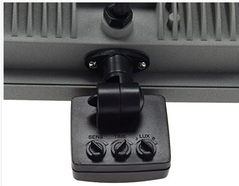
Figure 7.1: The three adjustment knobs on the motion sensor: SENS (Sensitivity), TIME (Duration), and LUX (Twilight Threshold).
