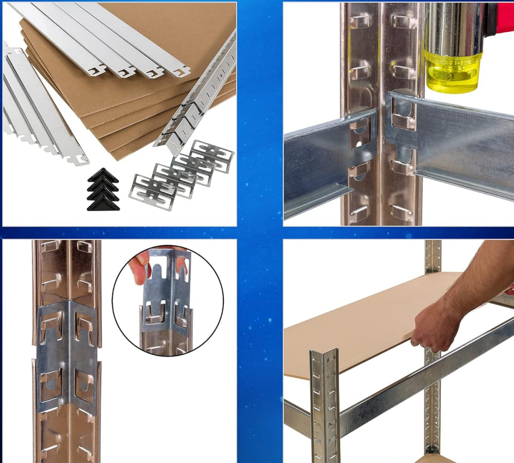
Image 3.2: Visual guide demonstrating the tool-free plug-in assembly process.
