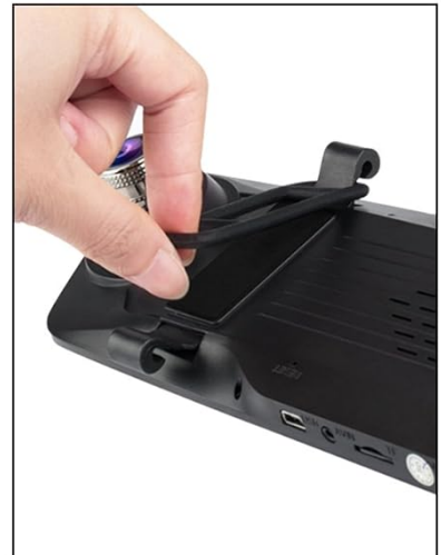
Image 4.1: Visual guide for attaching the dash cam to the rearview mirror using rubber straps.
