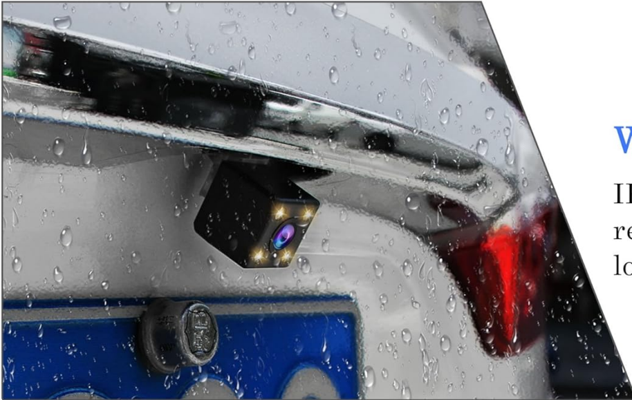
Image 3.2: Depiction of the waterproof rear camera and its parking assistance feature with guide lines.
