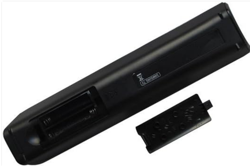
Figure 2.1: Rear view of the remote control with the battery cover removed, illustrating the battery insertion points. Two AAA batteries are required.
