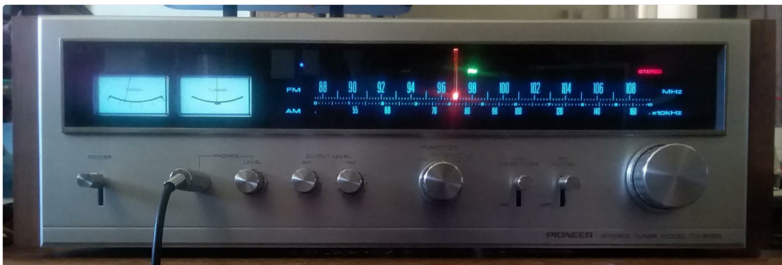
Image 3.2: A Pioneer TX-8100 Tuner after LED bulb installation, showcasing even and warm illumination.
