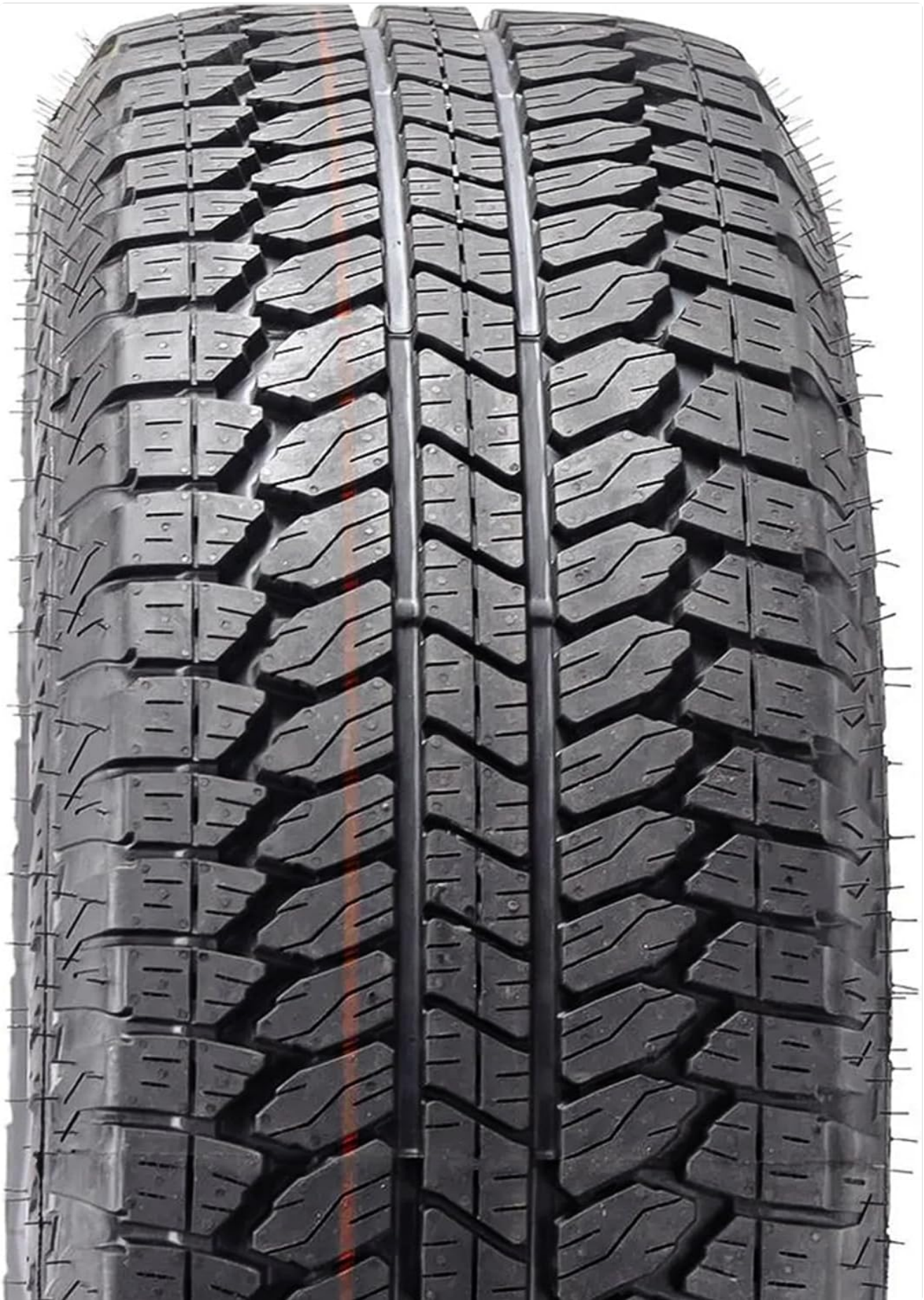
Figure 4.1: A detailed view of the Bridgestone Dueler A/T RH-S tire tread pattern, showing the aggressive blocks and grooves designed for all-terrain performance.
