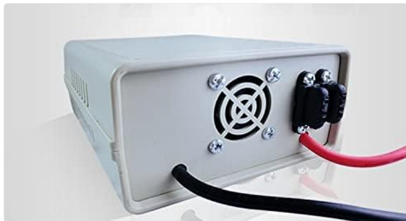
Image 4: Rear view of the device, clearly showing the cooling fan for heat dissipation and the power input terminals.
