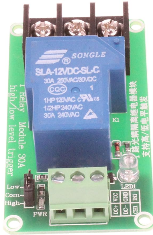
Figure 2: Close-up view of the relay module showing the input and output terminals. The VCC, GND, and IN1 pins are visible on the left, while the COM1, NO1, and NC1 terminals are on the right.
