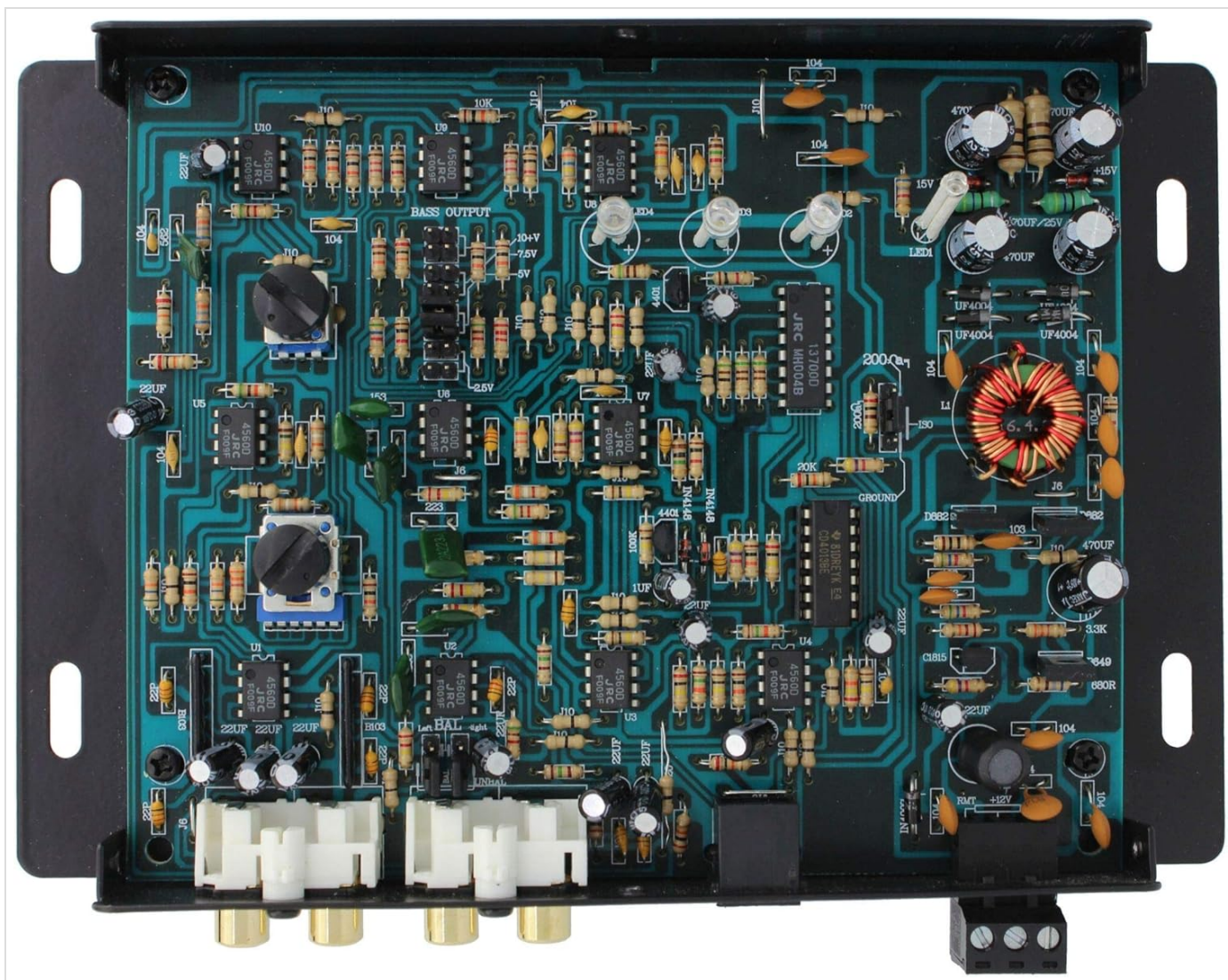
Figure 5: Internal view of the MEMBX Bass Expander's circuit board, showing various electronic components. This view is for informational purposes only; users should not open the unit.
