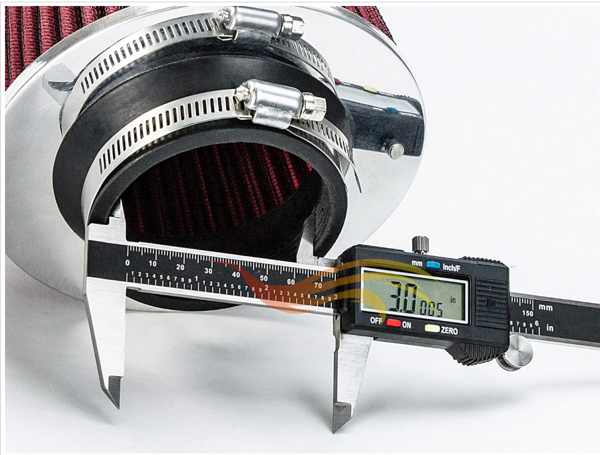
Figure 2: Detailed dimensions of the air filter, including its 3-inch inlet diameter, 5.25-inch height, and 6.25-inch base width.
