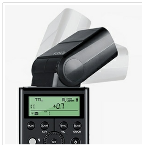
Figure 4.4: The flash head can be tilted to various angles for bounce lighting.
