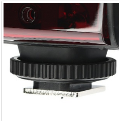
Figure 3.2: The hot shoe connection point on the flash unit.
