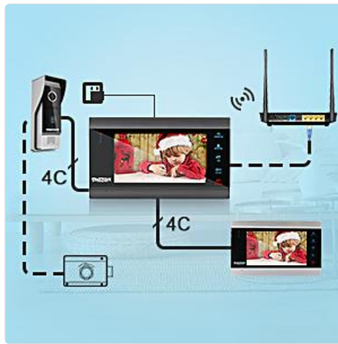
Image: Comprehensive diagram showing how the doorbell, master monitor, slave monitor, and Wi-Fi router are interconnected.
