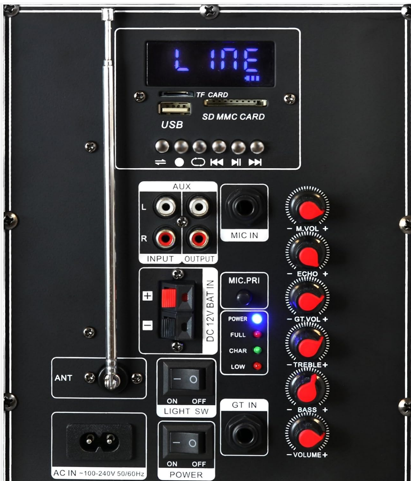
Figure 3.3: Detailed view of the rear control panel, featuring USB/SD/TF card slots, AUX inputs/outputs, microphone and guitar inputs, volume controls, echo, treble, bass adjustments, and power/light switches.
