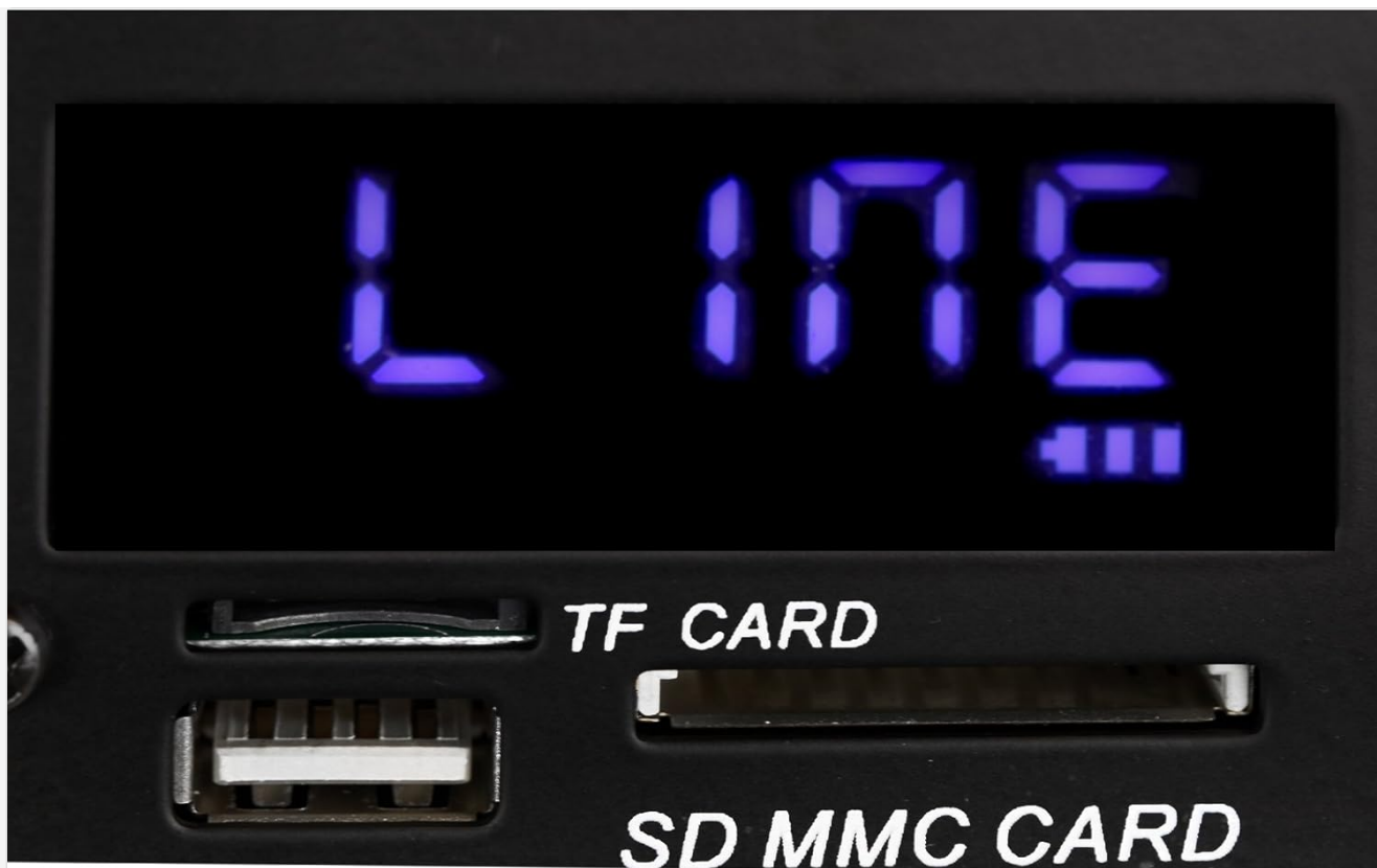
Figure 3.4: Close-up of the digital display showing 'LINE' mode, along with the USB port, TF card slot, and SD/MMC card slot for media playback.
