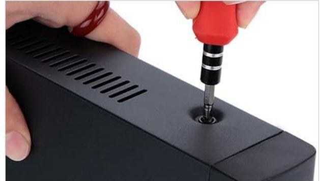
Figure 3.1.1: Visual guide for installing the hard drive, showing the process of opening the DVR, connecting cables, and securing the drive.
