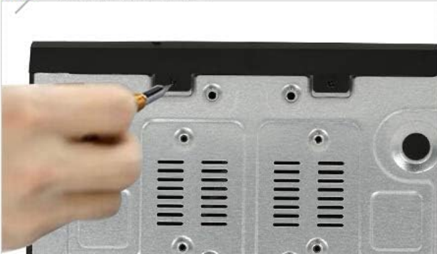
Figure 3.1.1: Visual guide for installing the hard drive, showing the process of opening the DVR, connecting cables, and securing the drive.
