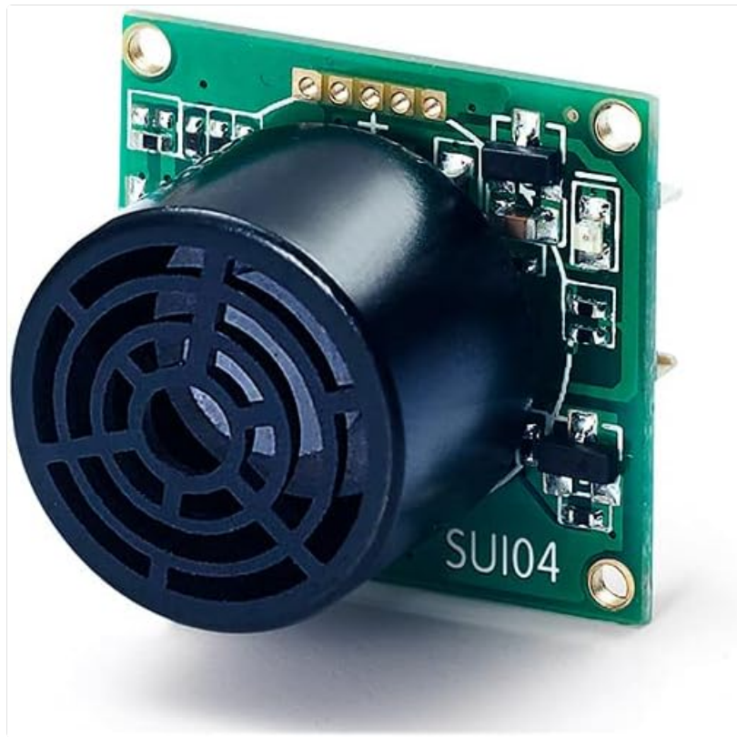
Image 1.1: The Radiolink SUI04 Ultrasonic Sensor module, showing its compact design and transducer.
