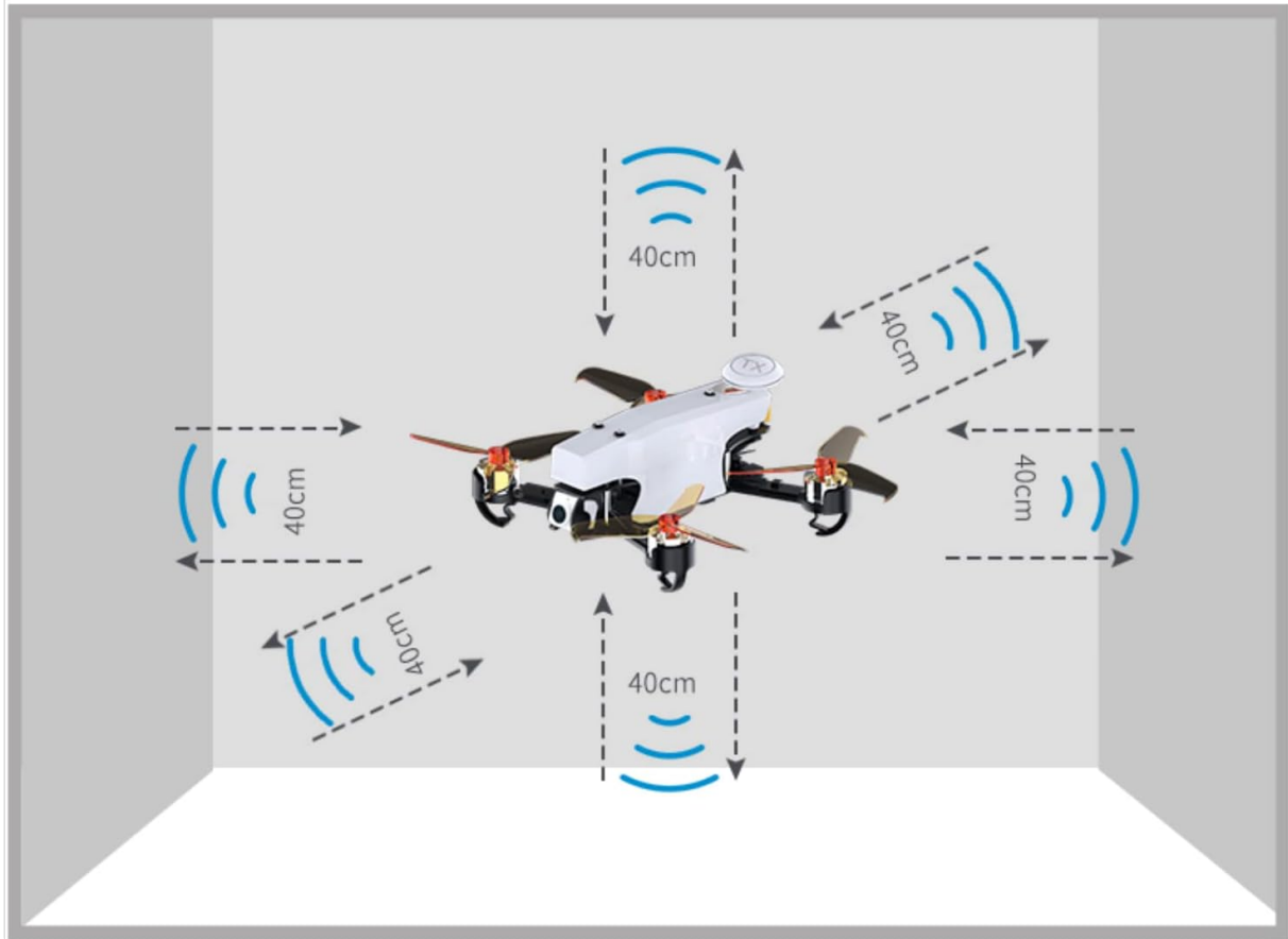
Image 3.2: Diagram showing a drone utilizing SUI04 sensors for obstacle avoidance in six directions.
