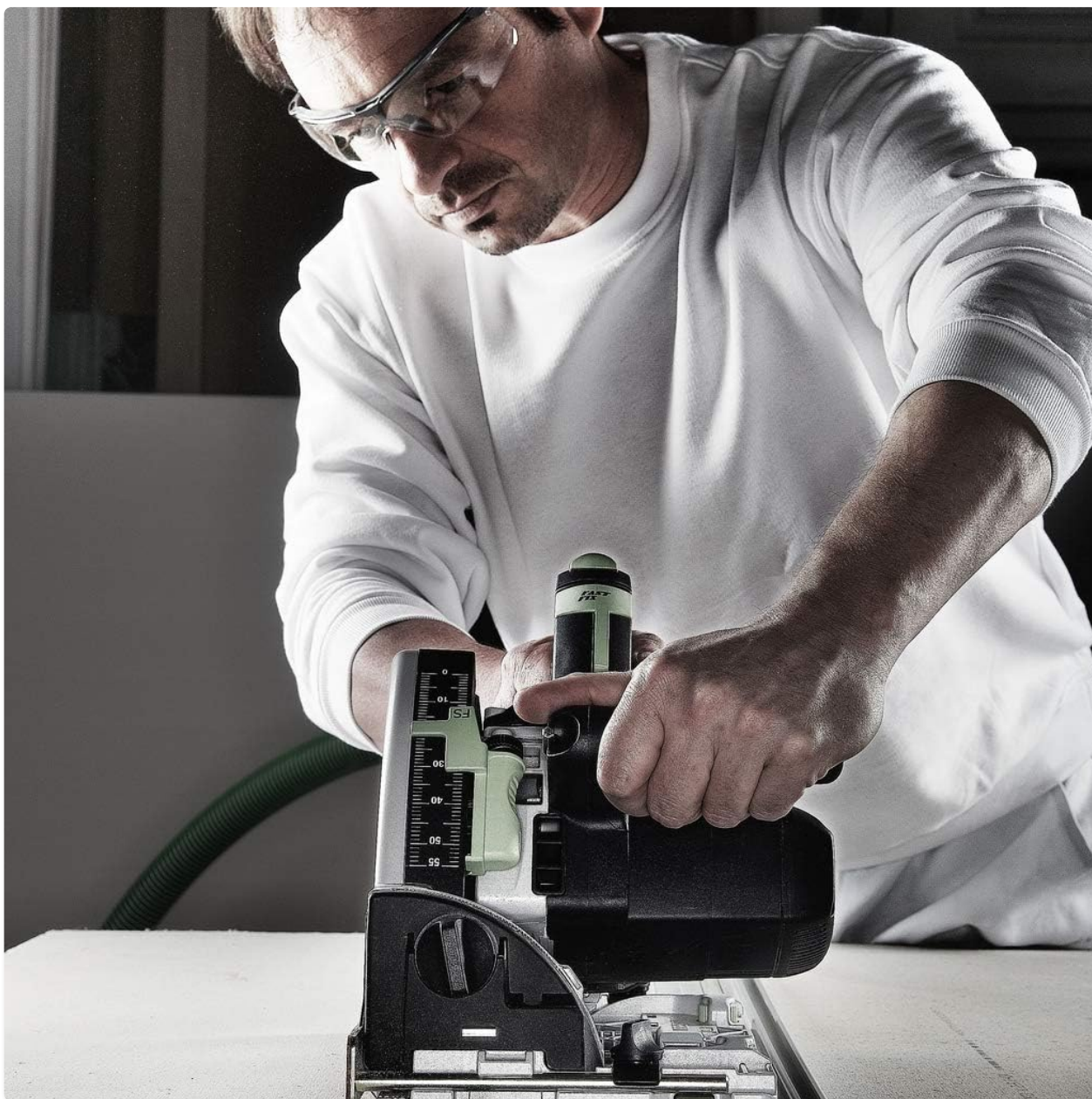
Image: A user adjusting the settings on the Festool TS 55 REBQ Plunge-Cut Saw, likely for depth or bevel angle.
