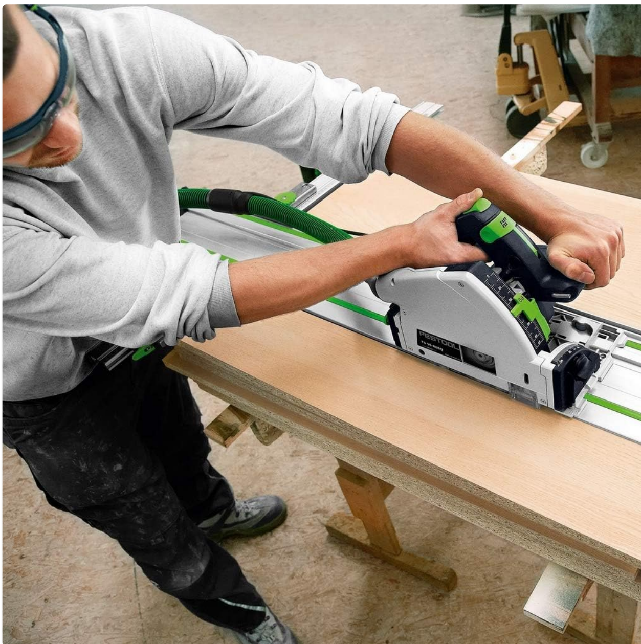
Image: A user demonstrating the use of the Festool TS 55 REBQ Plunge-Cut Saw with a guide rail on a wide wooden panel.
