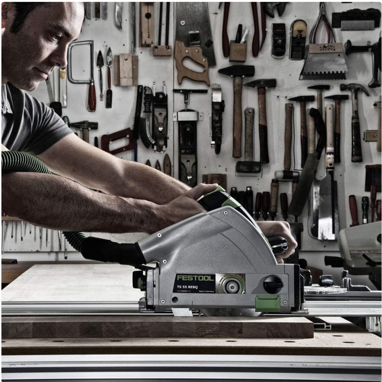
Image: A user operating the Festool TS 55 REBQ Plunge-Cut Saw, connected to a dust extraction hose for a clean work area.
