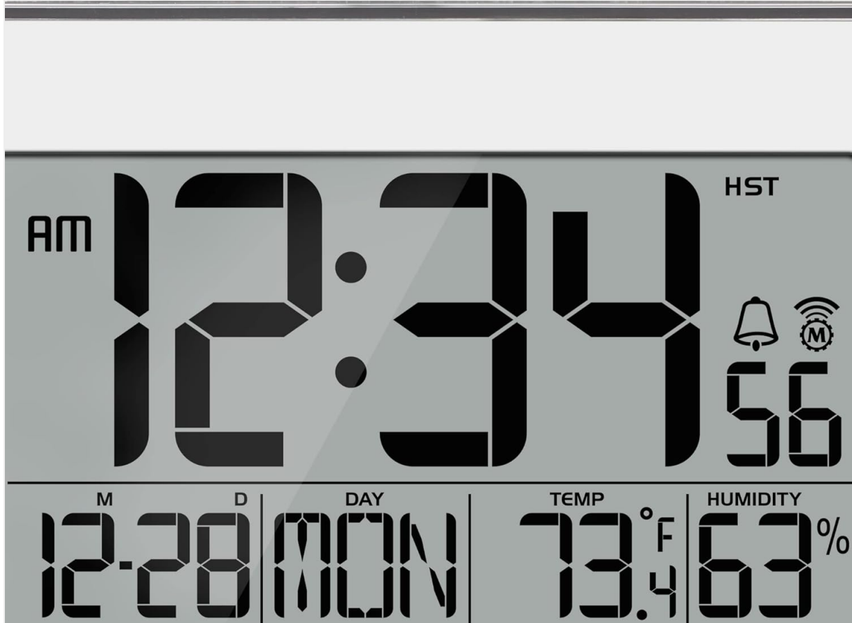
Image: A detailed view of the clock's dynamic display, illustrating the simultaneous presentation of time, date, day of the week, temperature, and humidity.
