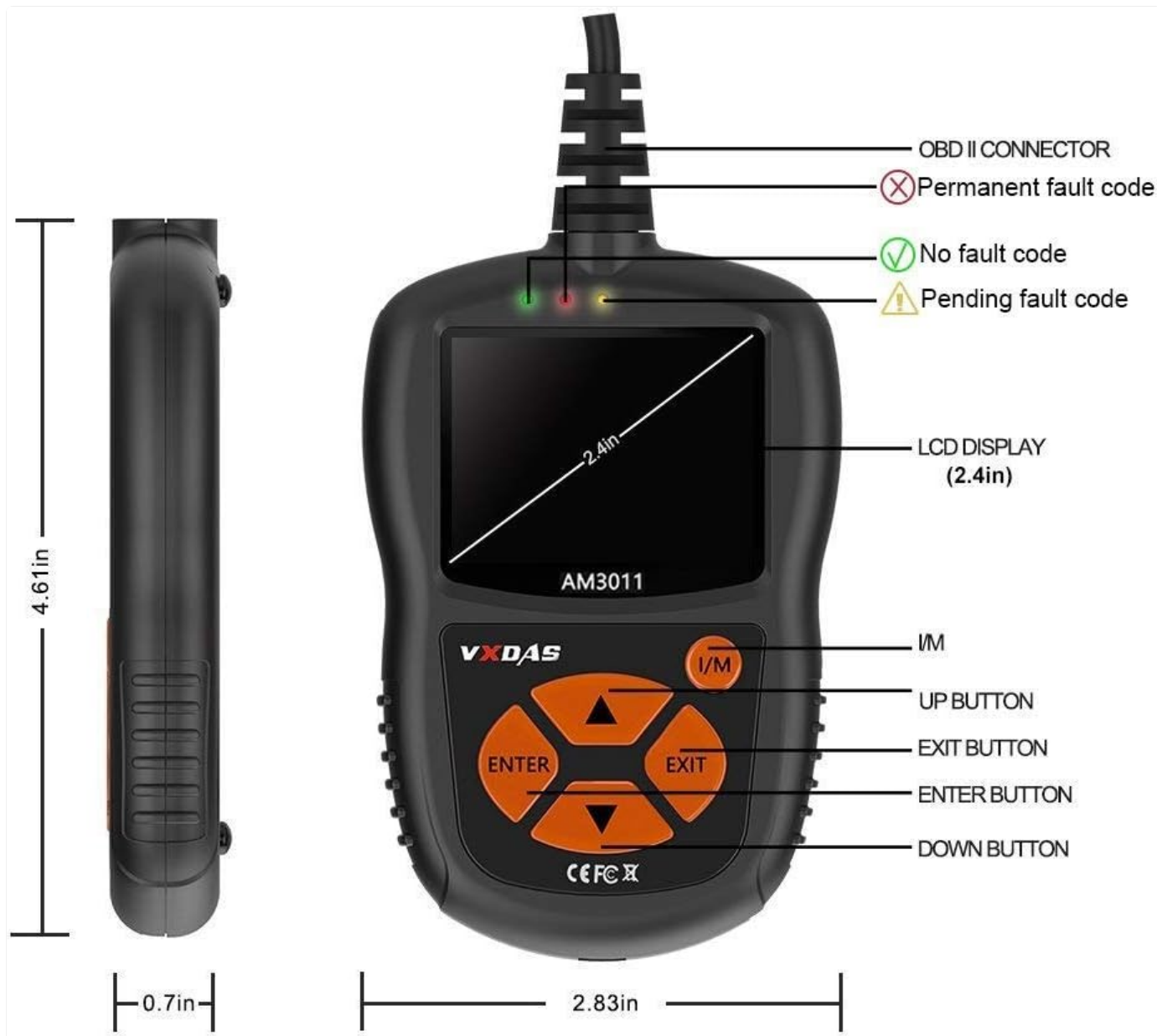
Figure 5: A diagram illustrating the physical dimensions of the VXDAS AM3011 scanner, including its length, width, and thickness, along with the 2.4-inch LCD display size and button layout.
