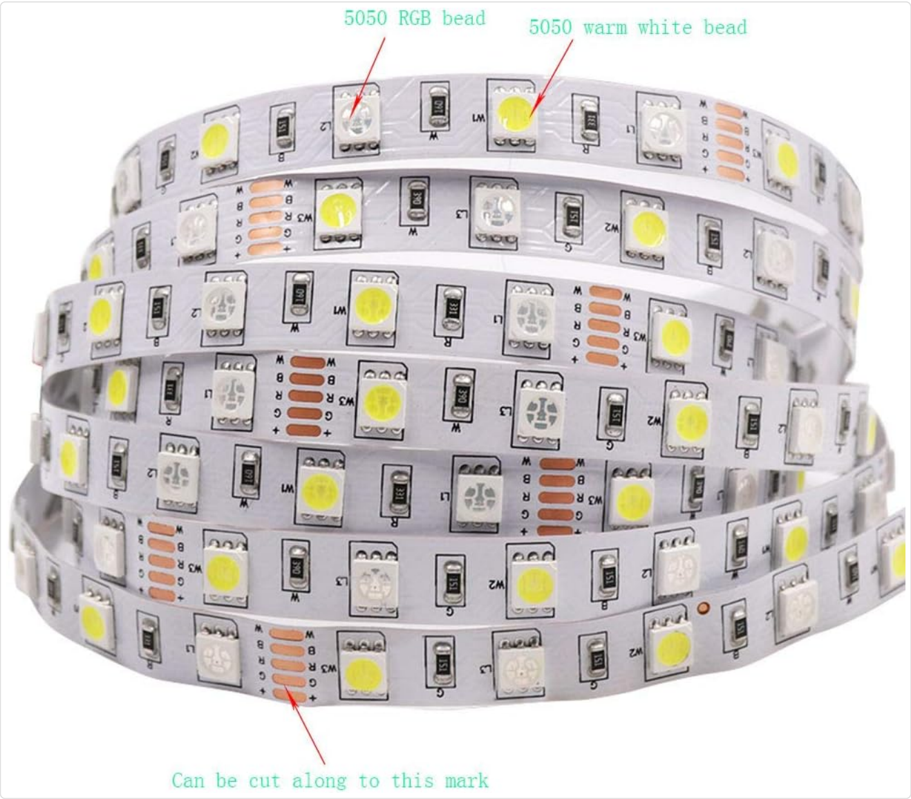
Image 4.1: Close-up view of the LED strip, highlighting the 5050 RGB and warm white beads, and indicating the safe cutting points along the strip.
